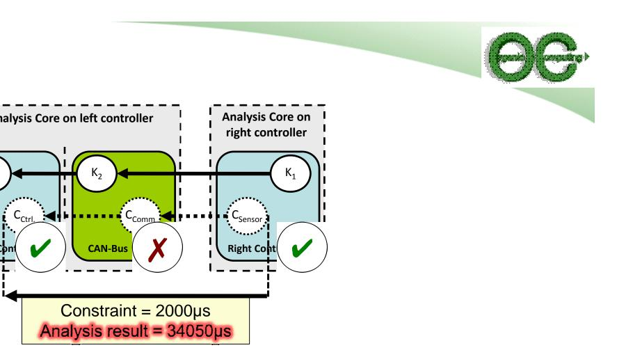
The third application would cause the control application to fail its latency constraint. The third application is rejected.
