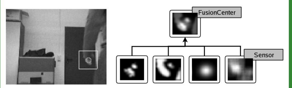
Tracking agent in use, on the left we see the tracking result marked with the circle. The rectangle shows the border of the agent's search region. On the right we see the similarity maps created by the different sensors, from left to right: color, motion, motion prediction and pixel template. The fusion center shows the result of the information integration.
