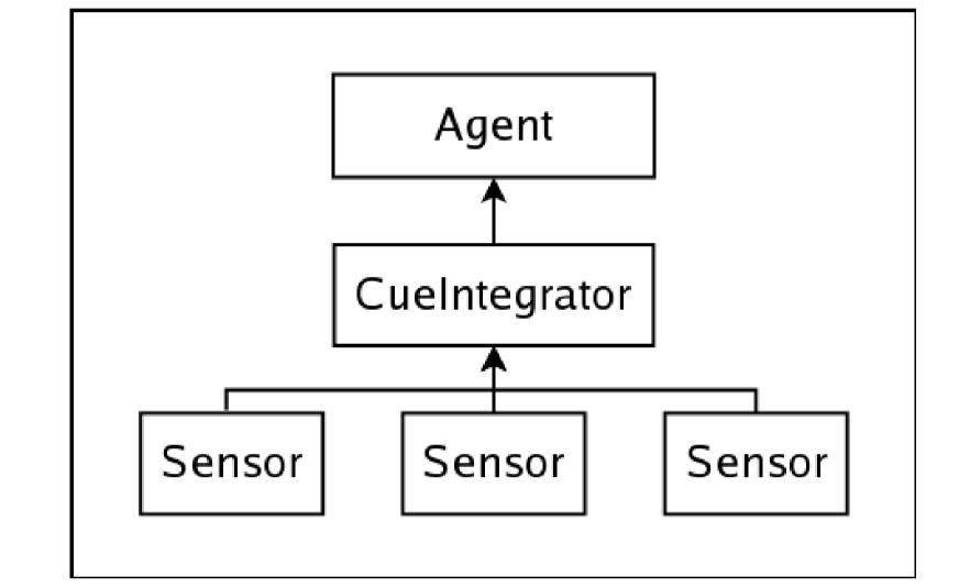
An agent is based on three modules provided with as much flexibility as possible. The interface to the environment and the communication are included in the agent class. Then there is one cuelntegrator, the module that integrates and interprets the information provided by the sensors.
