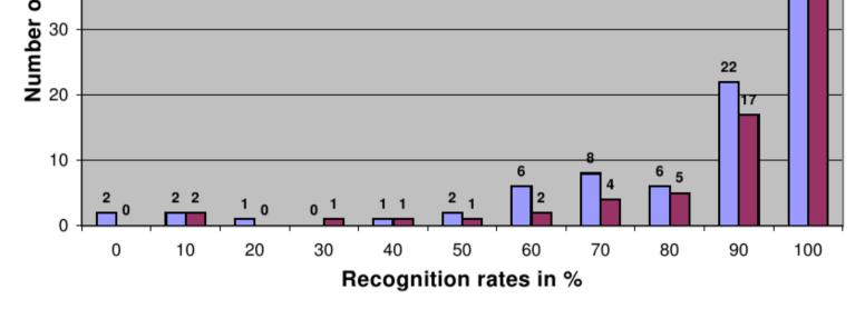
Recognition started with the beginning of the gesture. The histogram shows the result for the experiment using only position and contour information in light color and in dark color the result when integrating position, contour and texture information.
