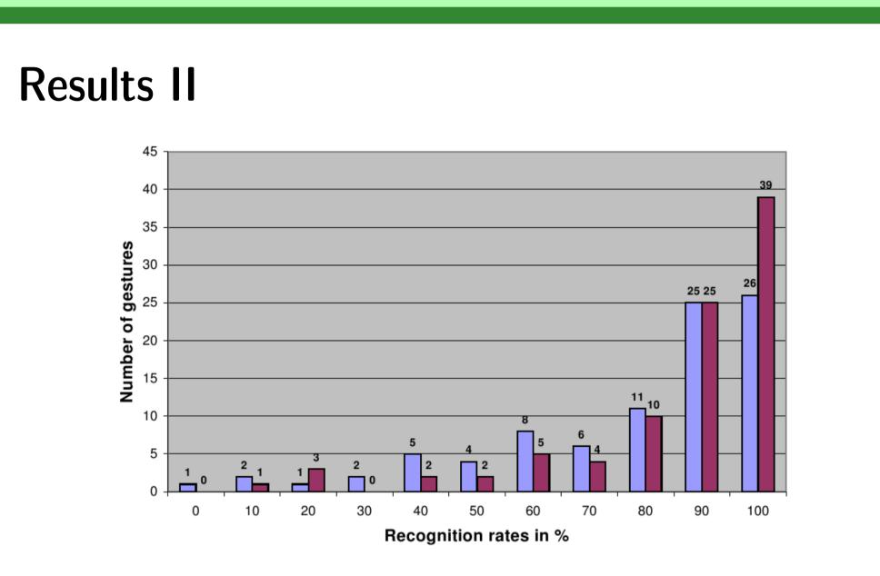
Recognition started 10 frames before the beginning of the gesture to examine the effect of co-articulation. The histogram shows the result for the experiment using only position and contour information in light color and in dark color the result when integrating position, contour and texture information.
